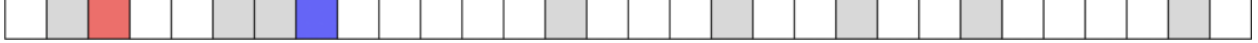
Figure 1: Samples of a codeword in vanilla FRIDA. Grey squares denote non-interactive samples common to both nodes ( L = 9 ). Red squares denote the Q = 1 sample from the first light node, while blue squares denote the Q = 1 sample from the second light node.
