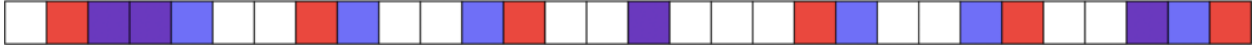
Figure 2: Samples of a codeword in interactive FRIDA. Red squares denote samples held only by the first light node, blue squares denote samples held only by the second light node, and purple squares denote samples held by both nodes.
